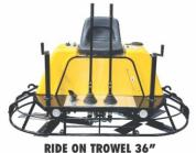
**SPRT-236B HIGH RIDER** Model- Trowel Machine Engine- Honda GX690 Working Dia- 1980mm Max Speed- 150rpm Tank- 15L, Weight- 350Kg
